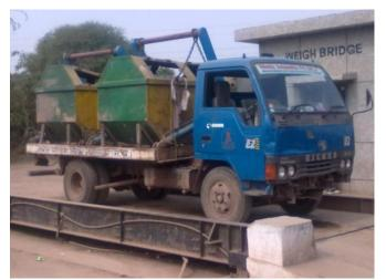
In processing plant, firstly the received waste weighed on Weigh Bridge of 25 ton capacity. Records of received waste maintained regularly. Received waste contains 30% inert, 20-25% Refuse-derived fuel (RDF), 15% compost & 35% inorganic. Plastics, rubbers,
