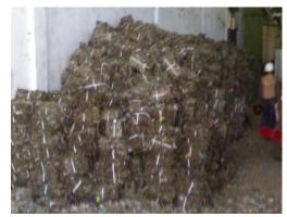
Refused derived fuel (RDF) contains 4-5% of 7,000-8,000 Calorific values plastics, 90% paper, organic matters and woods etc. Samples of RDF send to in house laboratory to calculate calorific value. The flow chart of RDF preparation is given at *Annexure* – *II*. The each packet of RDF has
